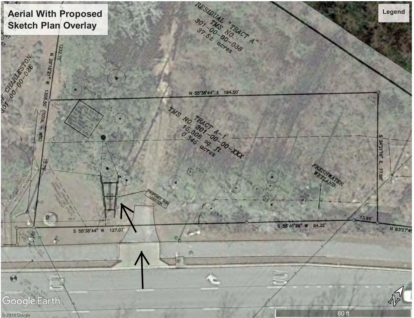
Construction/vehicular entrance will use existing curb cut
