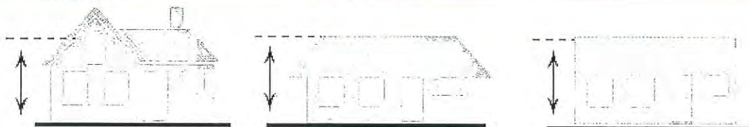
Gable, Hip, or Gambrel Roof Mansard Roof Flat Roof
