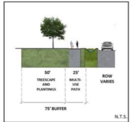
FIGURE 1 RIGHT-OF-WAY BUFFER, MAIN ROAD
